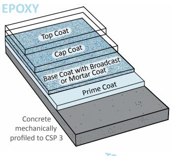
Traditional single-broadcast epoxy system at 1/8" thickness.
